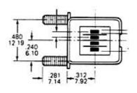
TWO 2-56 STUDS (On side of spring clip.) QK-18 "SE" Erase Heads QK-20 "G" Size R/P Heads QK-38 All "B" Size Heads
